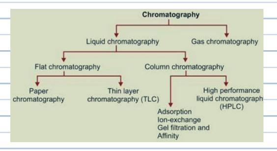
All chromatographic techniques consist of a stationary phase and a mobile phase.
